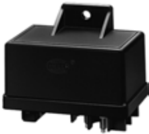
12 V, no. of poles 9, preheating time at +20°C / < 8 sec, Terminal S = postheating cut-out 4RV 008 188-321 Citroën, Peugeot
