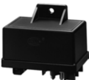
12 V, no. of poles 6, preheating time at +20°C / < 8 sec 4RV 008 188-301 Citroën, Fiat, Peugeot
